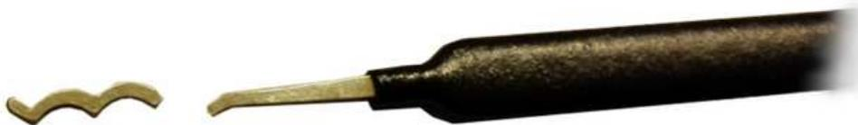
**Important Note:** Be careful with your tension wehn raking. While you can get away with heavier tension during single pin picking, too much tension while raking can result in a broken pick.
