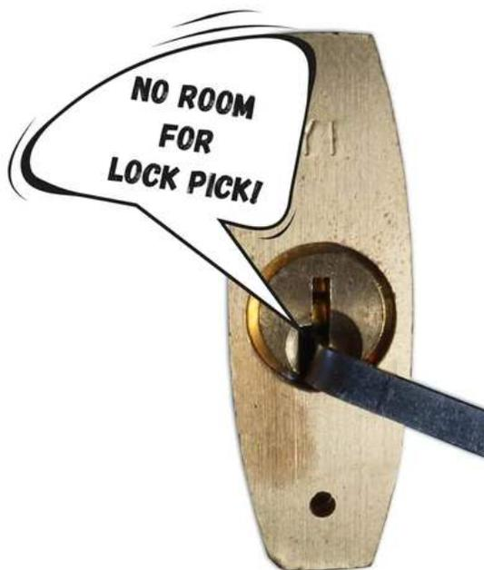
Secondly, when we move our tensioning tool from BOK to TOK, we create a LOT more room in the keyway to maneuver and leverage our picks.
